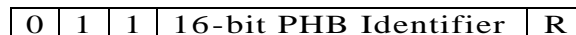
Figure 4: Binary format for 20-bit flow label field in IPv6 base header [44, Banerjee 2002]
