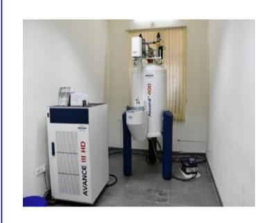
Applications: i) Analysis of 1D NMR: Proton |i) Measurement of specific (19F), Phosphorus (31P). ii) Analysis of 2D NMR: (ii) Measurement of pore size, COSY, NOESY, HMBC, pore volume and pore size HSQC.
