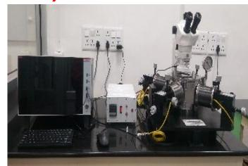
Applications: Advanced measurement hardware for DC I-V, C-V, and pulsed I-V measurement types.
